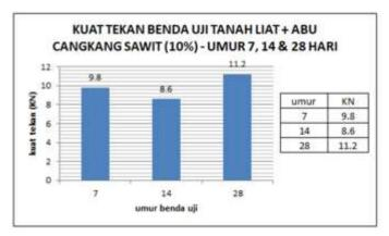
Gambar 3.17: Kuat Tekan Benda Uji Tanah Liat + Abu Cangkang Sawit (10%) – Umur 7, 14, 28 Hari
