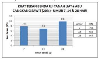
Gambar 3.20: Kuat Tekan Benda Uji Tanah Liat + Abu Cangkang Sawit (20%) – Umur 7, 14, 28 Hari
