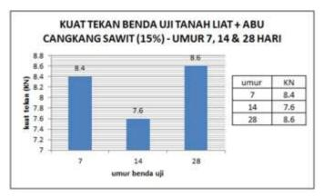
Gambar 3.19: Kuat Tekan Benda Uji Tanah Liat + Abu Cangkang Sawit (15%) – Umur 7, 14, 28 Hari
